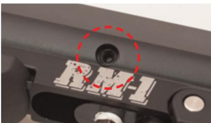
6. To increase or decrease the velocity of the paintballs discharged from a marker, use a 5/32" allen wrench to turn the screw clockwise to reduce velocity and counterclockwise to increase velocity. Note: When adjusting the velocity, make small adjustments, testing after each
