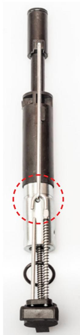
**IMPORTANT:** When reassembling the marker, make sure cocking rod (15) is hooked to connecting rod (13) correctly or marker will not cycle.
