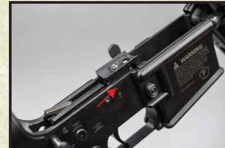
Remove upper manifold by pushing the small pin
