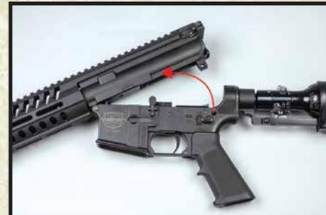
Remove rear receiver pin and pivot upper receiver forward
