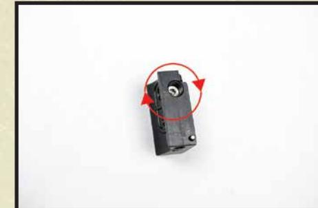
Adjust the velocity screw with a 3/32" allen
