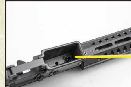
Use airsoft safe silicone to lubricate the hop up chamber. Use sparingly.
