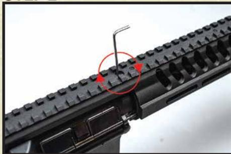
To increase the hop up setting, rotate the hop up dial with a 7/64" allen (Clockwise) towards hop.
