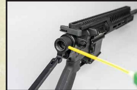
Use airsoft safe silicone to lubricate the asa
