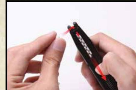
1. Pull the magazine feed spring down and hold.
