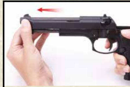
Pull the slide forward to separate from the gun and expose the hop up adjustment.
