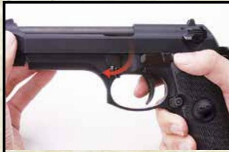
Turn the slide release lever to release mode.
